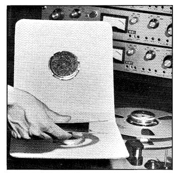
FIGURE 11. IMPROPER HANDLING OF TAPE REEL. SQUEEZING THE FLANGES MAY CREATE SERIOUS TAPE DAMAGE.
