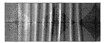
FIGURE 6. TAPE DAMAGE CAUSED BY CINCHING.
