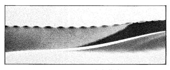
FIGURE 8. SEVERE EDGE DAMAGE.
