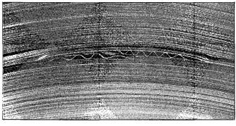
FIGURE 5. CINCHED TAPE, NOTICE DISTORTION OF TAPE LAYERS.
